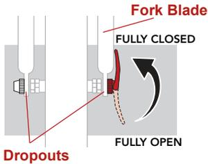
While maintaining the wheel in this position, rotate the quick release upward and into the FULLY CLOSED position. When properly closed, the curve of the quick release will be pointing toward the wheel and parallel to the fork blade. To generate enough clamping force it is necessary to wrap your fingers around the fork blade while closing the quick release lever. The proper force required to close the quick release lever should leave a visible imprint in the palm of your hand.
