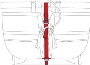
Centre Tension Strap provides support for the centre of the seats and positions the Centre Mount for the canopies. It comes pre-adjusted from the factory; however it can also be tightened if necessary. Tighten this strap to keep the seats from leaning toward each other.
