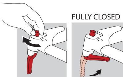
To properly close the quick release and secure the rear wheel in the dropouts, confirm the axle is fully inserted in the dropout, while maintaining the wheel in this position, rotate the quick release toward stroller and into the FULLY CLOSED position.
